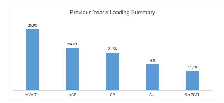
The Non-coincident Peak Demand is 24.28 MW, which is around 69.37% of the total substation capacity of 35MW. The load factor or the ratio between the Average Load of 14.91 MW and the Non-coincident Peak Demand is 61.40%.
